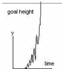
Fig. 3. Acrobot Swing-Up Problem: vertical position versus time
