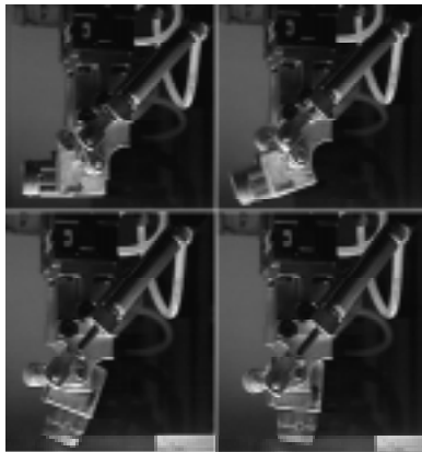
Figure 4: Rotary Jaw Gripper in Action
